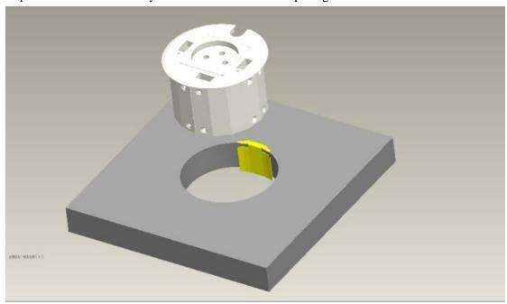
Step 4. Adjust slightly the main body position to match its cable slot to the metal piece properly:
