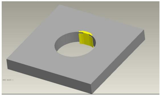
Step 3. Insert the main body of JXH-3U90-IL into the opening hole:
