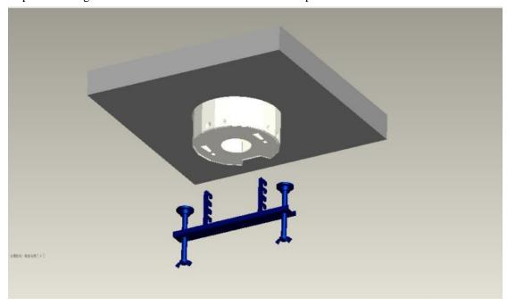
Step 6. Fasten the installation bracket:
